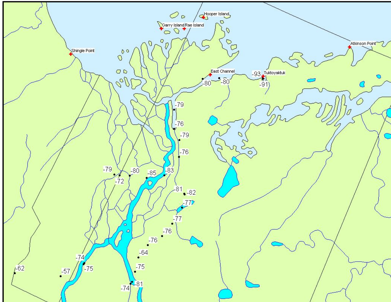
Figure A.6: Difference between the leveling datum of Nov04 and geoid datum of CGG05 at benchmarks in the region of the Mackenzie Delta. The discrepancy is determined by h - H - N where h is the ellipsoidal height in ITRF2000 measured by GPS, H is the orthometric height (Nov04) and N is the geoid height (CGG05). The discrepancies are expressed in cm.
