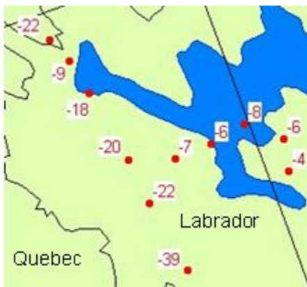
Figure 5: The 13-cm step between the NS and EW levelling lines in Labrador
